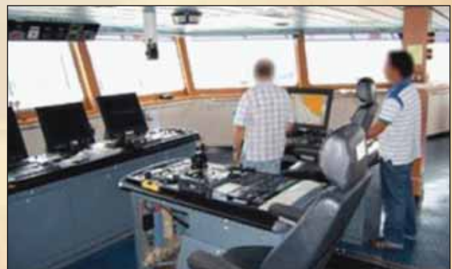
View of bridge showing the offset location and athwartship orientation of ECDIS display.
